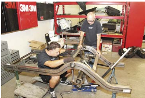
■ The Chris Alston Chassis Works FAB9 rear axle housing and canted 4-bar rear suspension was assembled to the Chris Alston Chassis Works back-half frame clip.
