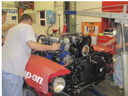
■ It was a tight fit to get the fully assembled big-block into the engine bay, but R&A Motorsports did it—just like Ford's San Jose plant did 46 years ago.
