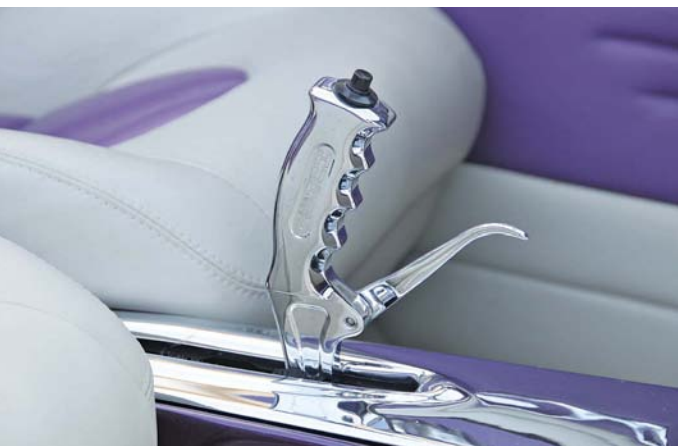
■ The Hurst shifter controls a GM 4L80E automatic transmission. The button on top is the reverse lock out.
