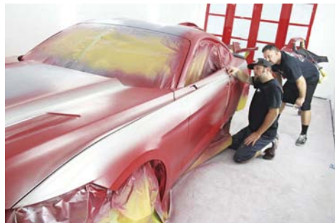
■ After spraying AXALTA Super Silver where pinstriping would be laid out, Andy and Casey eyeballed the straight and curved tapelines.
