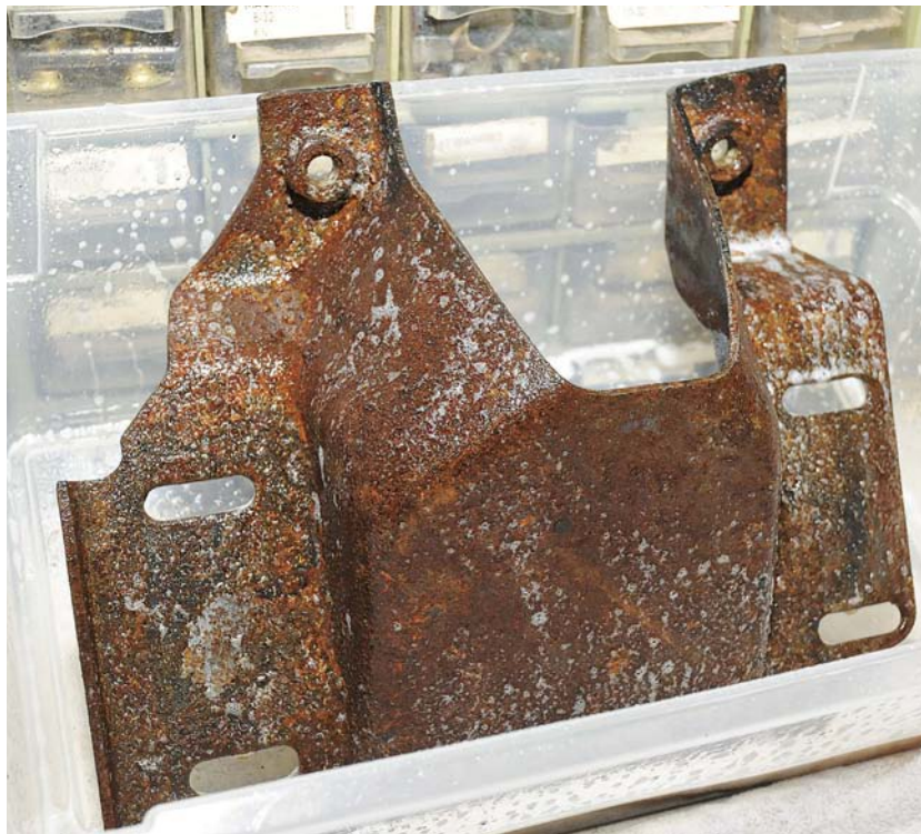
■ The front side gets the same treatment. Keep it wet with Metal Blast from the spray bottle.
