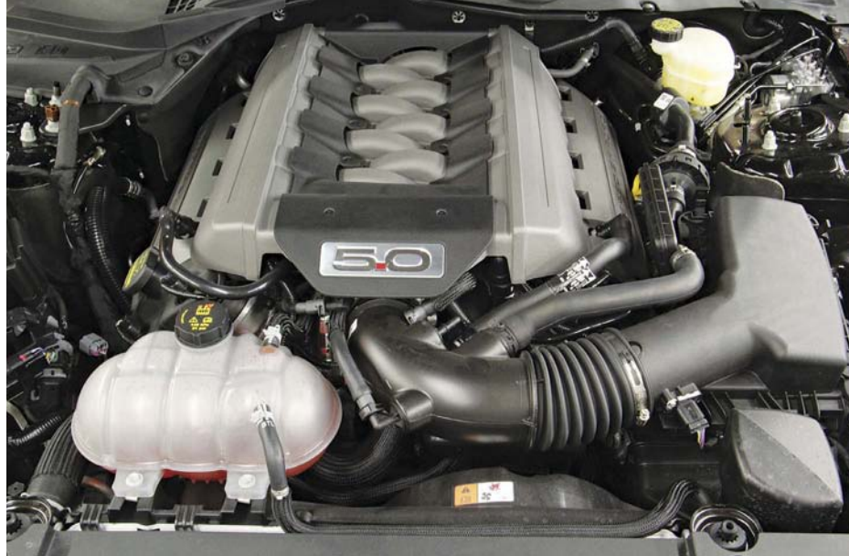
■ The factory Ford 5.0L V-8 Coyote engine was factory-rated at 435 bhp. That is about to be increased a whole lot.
