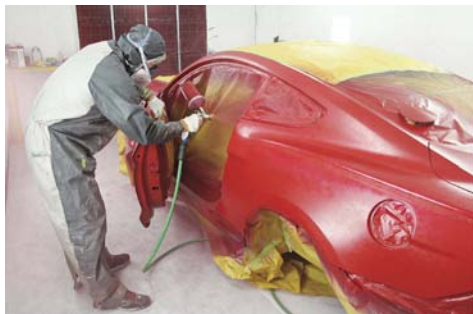
■ The body and door jams were then given color by spraying four coats of AXALTA CGS Red.
