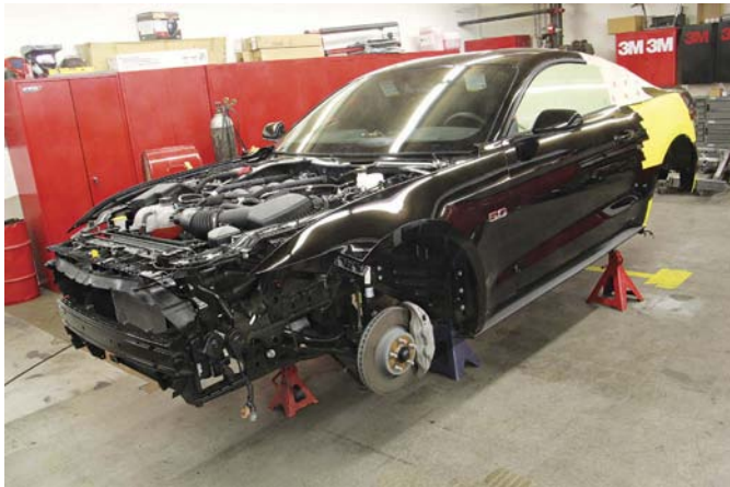
■ After the 2015 Mustang GT was delivered and the transportation papers signed, within minutes it was raised on jackstands and the wheels, hood, front grille, headlights and bumper cover assembly were all removed.
