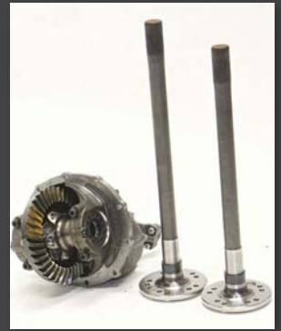
■ A Chris Alston Chassis Works FAB9 rear-end housing was gusseted for added strength to eliminate any axle tube flexing. Strange third member with 4.11 gears and a posi-unit was ready to bolt up to the FAB9 rear-end housing. A pair of Strange 35-spline axles was slid into the FAB9 rear-end housing to engage into the Strange third member gearset.
