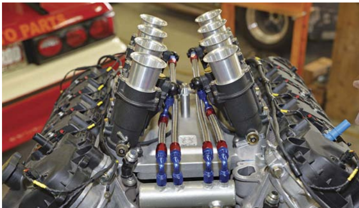
■ Now we are ready for the fuel system. We are installing the fuel manifold system for this particular engine because it will be used primarily on the race track. This is a parallel fuel system. This system is used to ensure that the last two injectors don't run lean, which is a possibility with the street setup under heavy use. All cylinders receive the same amount of fuel with the parallel fuel system.
