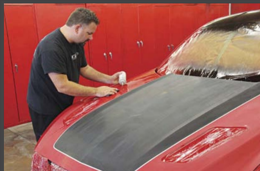
■ Casey wet-sanded every square inch of the freshly painted sheet metal using 3M products.
