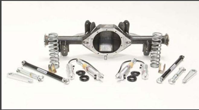
■ A Chris Alston Chassis Works FAB9 rear-end housing was gusseted for added strength to eliminate any axle tube flexing. Strange third member with 4.11 gears and a posi-unit was ready to bolt up to the FAB9 rear-end housing. A pair of Strange 35-spline axles was slid into the FAB9 rear-end housing to engage into the Strange third member gearset.
