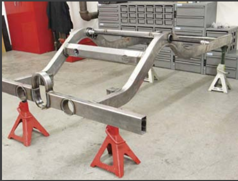
■ The Chris Alston Chassis Works weld-in, 4 x 2 rectangular tubing 4-link back-half, frame clip later would be fitted with Chris Alston Chassis Works rear suspension components.
