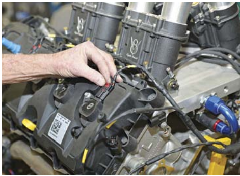
■ Hooking up the coils 5, 6, 7 and 8.
