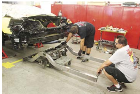
■ Casey and Robert Henry rolled the assembled Chris Alston Chassis Works back-half clip and suspension under the Mustang for preliminary fitment.
