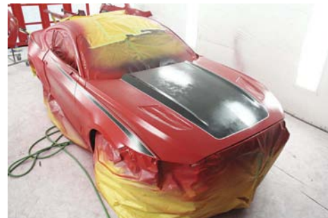
■ The hood center and scalloped areas were then painted with AXALTA Super Jet Black. Then the masking tape was removed.
