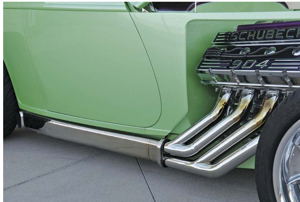
■ The oval tube exhaust was hand-built at Super Rides By Jordan.
