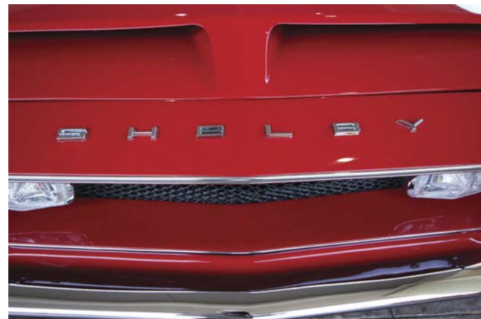
■ The chrome letters on the nose that spelled “Shelby” were closer together than on the production 1968 cars, so the spacing had to be determined by scaling the spacing using known dimensions in the photographs. DST built the front of the car as a single piece of hand-laid fiberglass. The 1968 production cars would have a 4-piece nose. It required close study of the factory photos that were eventually found to verify these details.
