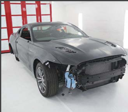
■ Time to paint. After removing grille, headlights/running lights, front and rear bumpers, door handles, gas tank filler door, hood vents, and other small body components, the Mustang was rolled into the CGS paint booth. The factory black exterior was scuffed using 3M pads and made ready for masking and sealer.
