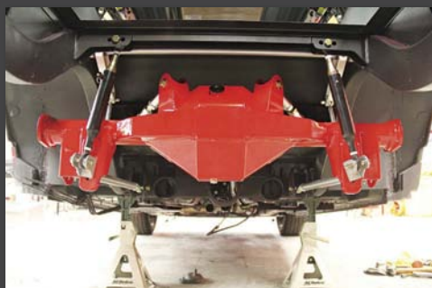
■ The Chris Alston Chassis Works FAB9 rear-end housing and 4-bar suspension were retrieved from Inland Powder Coating in Ontario, California, and reassembled. A pair of Speedway Motors adjustable mockup shocks were used to locate the FAB9 rear-end housing.
