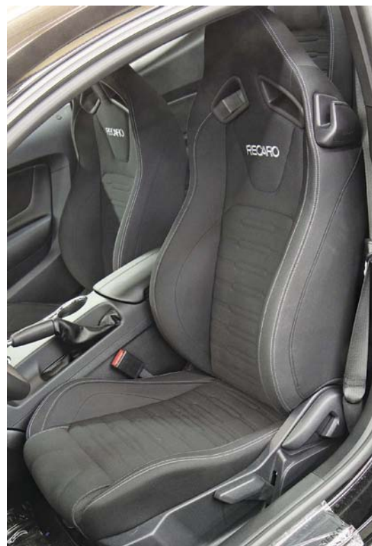
■ The team chose a pair of Recaro high-bolster racing bucket seats, with forward-back sliding rack, up-down action and tilt seatbacks featuring shoulder harness ports.
