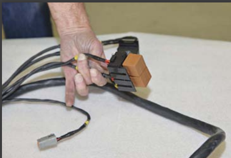
■ Hooking up the coils 5, 6, 7 and 8.
