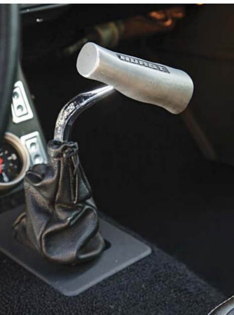
■ The shifter isn't a retro piece, but rather an old T-handle that had been laying around Herb's garage for decades. It's bolted to a Hurst gear lever.
