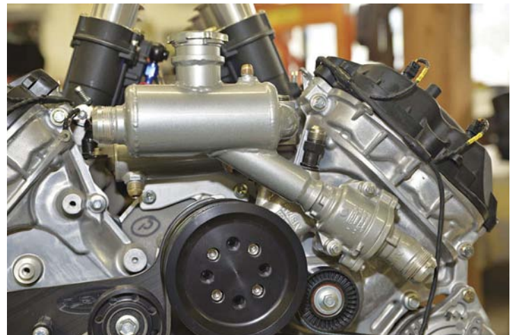
■ This custom application required a custom-built thermostat housing and expansion tank with the radiator service cap. It was fabricated by Merrell for the high-performance application, and it was necessary for fitting the Coyote engine in the Daytona Coupe for testing and tuning.
