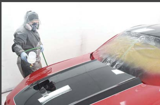
■ After wiping down the entire body, Andy began to apply the five coats of AXALTA Clear to achieve depth and glistening shine. The Mustang was left in the spray booth overnight to let the clear coats cure.
