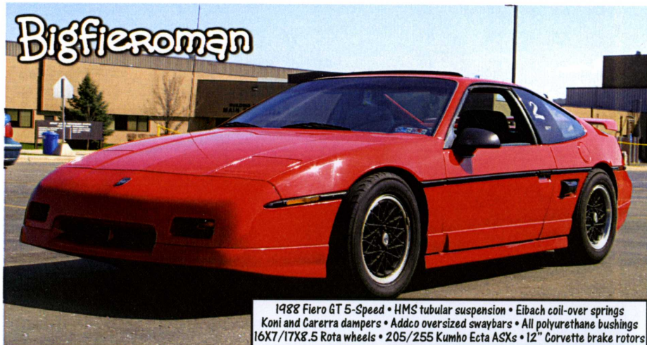
A V8 Archie built IRM IMSA coupe built on a 1988 Fiero Coupe. It has a ZZ4 350 CI TPI engine with a 5 speed getrag transmission. It has a PISA interior.
