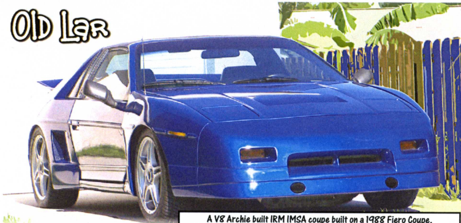
A V8 Archie built IRM IMSA coupe built on a 1988 Fiero Coupe. It has a ZZ4 350 CI TPI engine with a 5 speed getrag transmission. It has a PISA interior.
