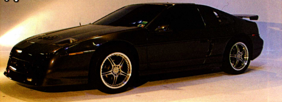
1988 GT- Charcoal Grey • 3800 Supercharged V6 • 5-speed Getrag Multiple Awards • 13.2 sec. 1/4 mile time • Poly / KYB's / 17's 12" Corvette Slot/Rotors • Custom Hood/ Bodywork
