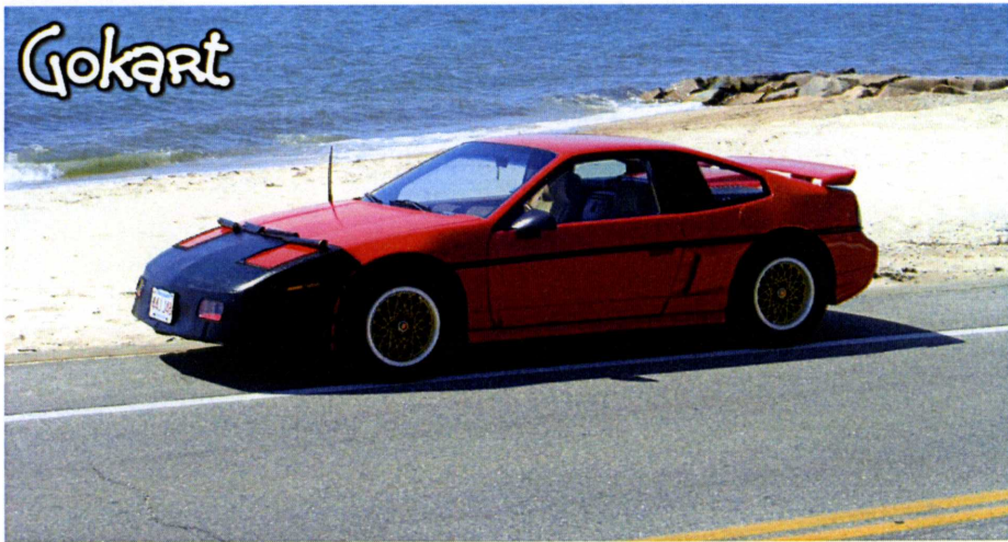
'88 Formula with Aldino • Kit Car body • 3800SC • 4T65E auto transaxle Fastest 1/4 mi street driven Fiero • 11.460 @ 110.77 mph 60 ft time 1.447 • Neatest looking, fastest Fiero! Still 23 mpg
