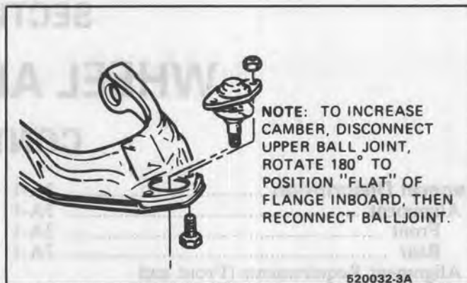
Fig. 1 Upper Ball Joint/Camber Adjustment (Front)
