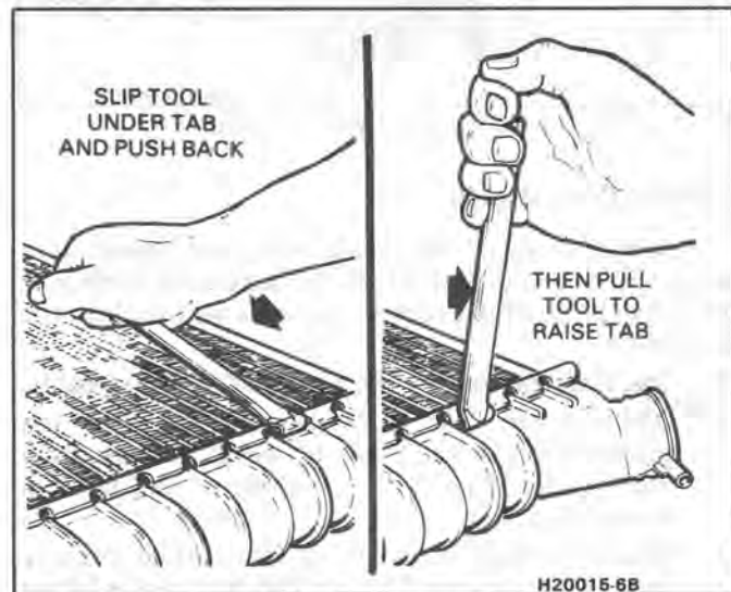
Fig. 23 Opening Clinch Tabs
