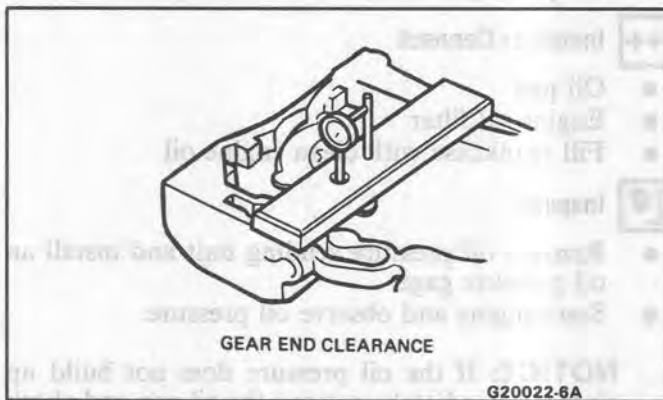
Figure 24 Gear End Clearance (Gear Drop In Housing)-Gerotor
