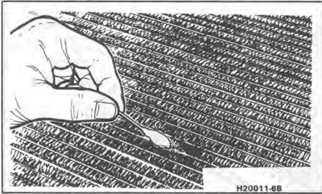
Fig. 19 Scrubbing Area with Primer
