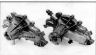
An aluminum V6/60 water pump housing can be modified to increase coolant flow by enlarging its inlet passage.
