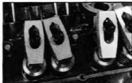
Check for interference between adjacent rocker arms when using aftermarket needle bearing rockers on V6/60 cylinder heads.
