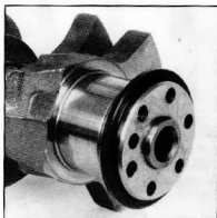
1985 and newer cranks with large 67mm main bearing journals and one-piece oil seals are recommended for competition V6/60 engines.
