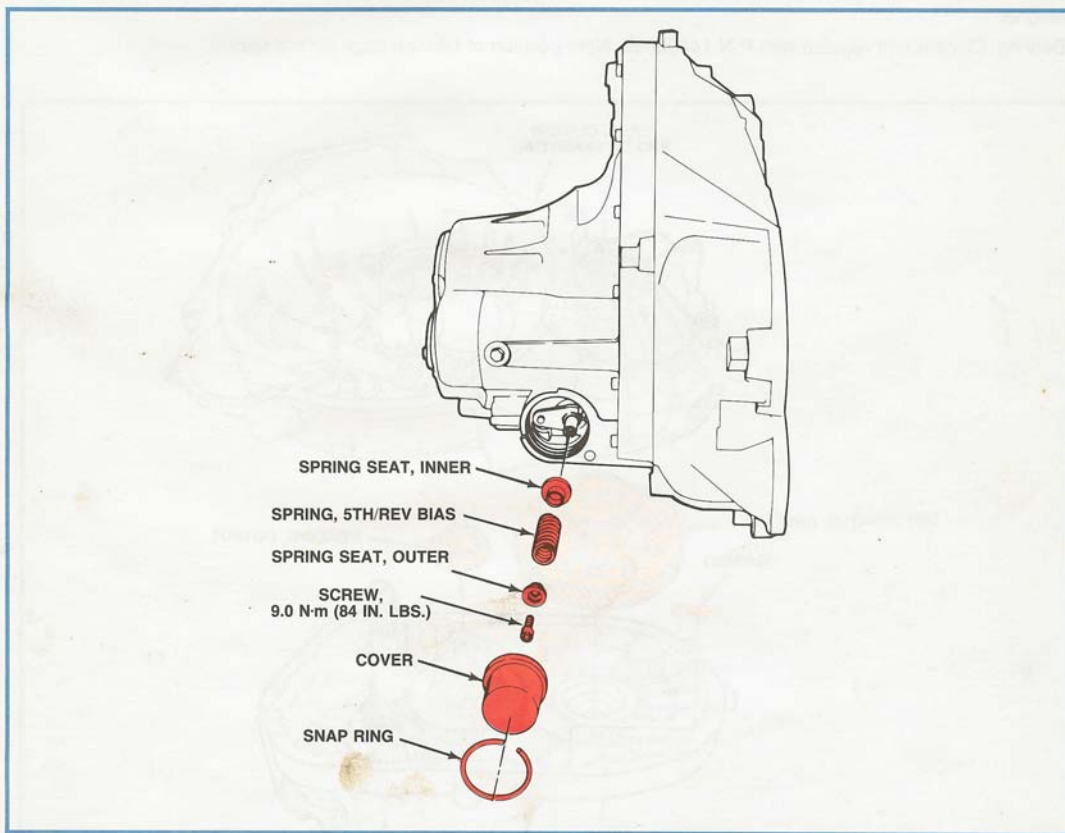
Figure 5-3, Shift Shaft Detent Components/Transmission Housing.
