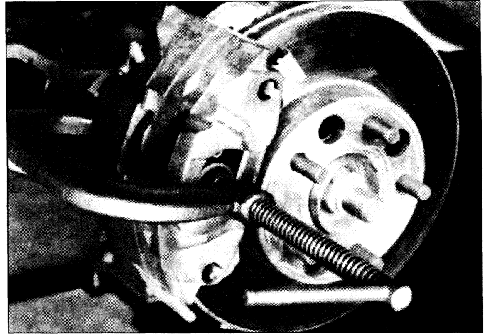
2.5 Use a C-clamp to push the piston back into its bore - tighten the clamp until the piston bottoms - as the piston is depressed to the bottom of the caliper bore, the fluid in the master cylinder will be pushed back into the reservoir (make sure it doesn't overflow)
