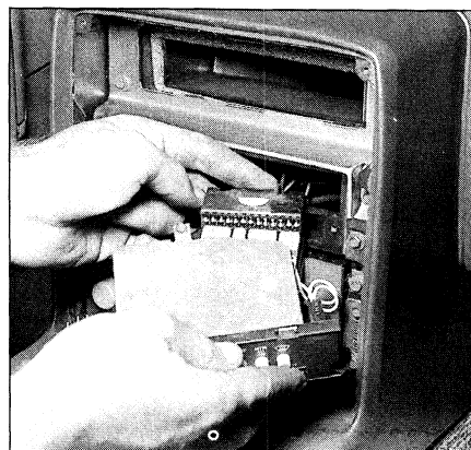
14.3b . . . then pull the heater control assembly out a little further and unplug the big electrical connector
