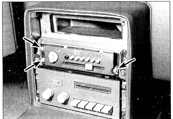
14.2 Remove these three screws (arrows) to pull out the heater control assembly
