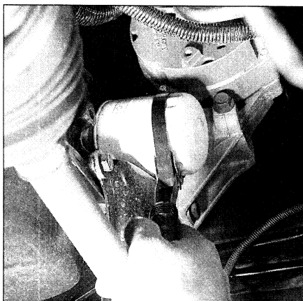
16.14 Use an oil filter wrench to remove the old filter - try to keep your hands away from hot engine parts and be prepared to catch some hot oil when the filter comes off
