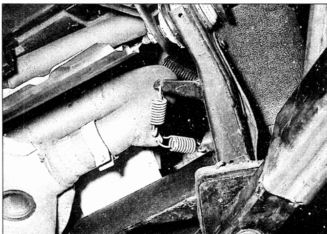
12.5 Remove the hanger springs from the left front corner of the cradle
