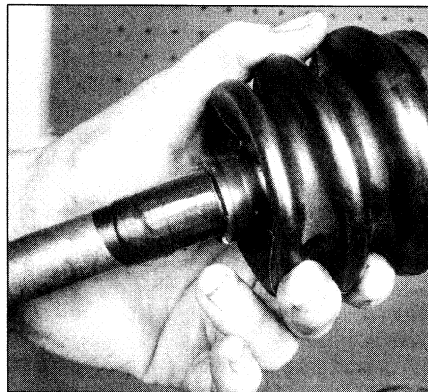
13.25b Wrap the axle shaft splines with tape to avoid damaging the boot, then slide the small clamp and boot onto the axle shaft
