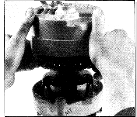
15.3a With the through-bolts removed, carefully separate the drive end frame and the rectifier end frame
