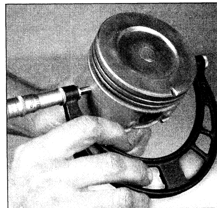
17.11 Measure the piston diameter at a 90-degree angle to the piston pin at the specified point on the skirt (see the Specifications)
