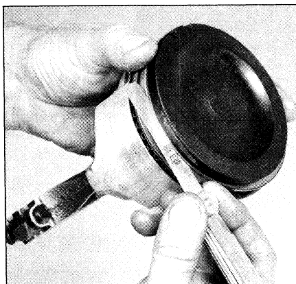
17.10 Check the piston ring side clearance with a feeler gauge at several points around the groove
