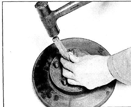
41.10 If either race is scored or galled, knock it out with a brass drift punch
