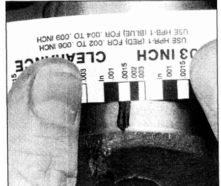
22.14 The crushed Plastigage is compared to the scale printed on the container to obtain the bearing oil clearance
