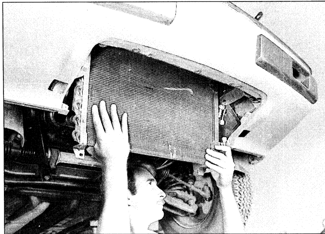
21.7 Removing the condenser from underneath the vehicle
