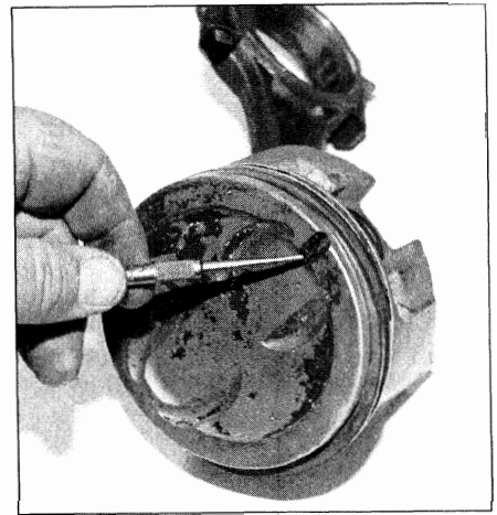
22.8 The notch or arrow on each piston must face the front (drivebelt end) of the engine
