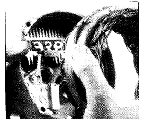
15.4 After removing the nuts holding the stator assembly to the rectifier bridge, remove the stator
