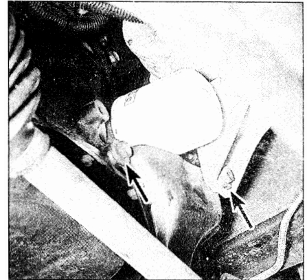
13.7b The rear mounting bolts for the front engine support bracket (arrows) - note that the bolt to the right of the oil filter is also a retaining bolt for the lower alternator bracket
