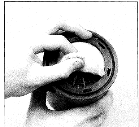
8.9 If the filter on the bottom of the canister is dirty, replace it with a new one
