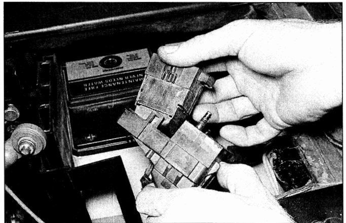
17.14b Disconnect the two-part plug from the junction box, then unplug the two sections of the plug from one another
