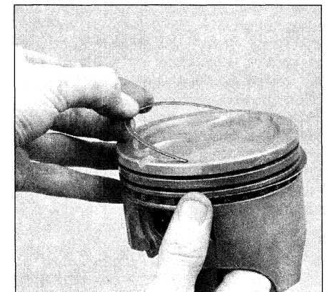
20.9b Do not use a piston ring tool when installing the oil ring side rails
