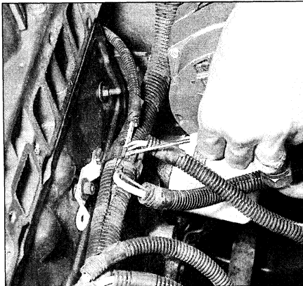
6.3 Disconnect the wire harness clip and push it out of the way to get at the pushrod cover retaining nuts
